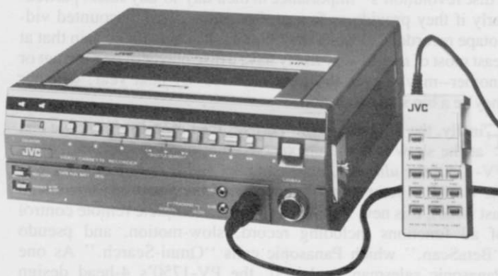
JVC's HR-2200U remote control consumer VHS portable features high-speed "Shuttle Search" cueing, frame-by-frame advance, and variable slow-motion.
