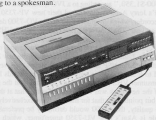
The "ultimate" consumer VHS recorder has to be Panasonic's PV-1750, offering full-function remote control and a 14-day/8-event programmable tuner.
