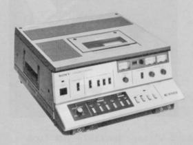
The specifications for this unit include: Signal/Noise ratio of 45 dB (color), horizontal resolution of 340 lines (B&W) and 240 lines (color), Audio S/N ratio of 45 dB, and audio frequency response of 50Hz to 10 KHz. The SLO-383 has full editing capability, direct drive, forward and reverse with fast and slow motion from 1/20 to 2 times normal speed in both directions. There is also Betascan at 8 times normal speed. The unit has
